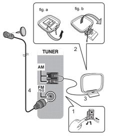
1 Push open the tabs, then insert one wire fully into each terminal, then release the tabs to secure the AM antenna wires.
