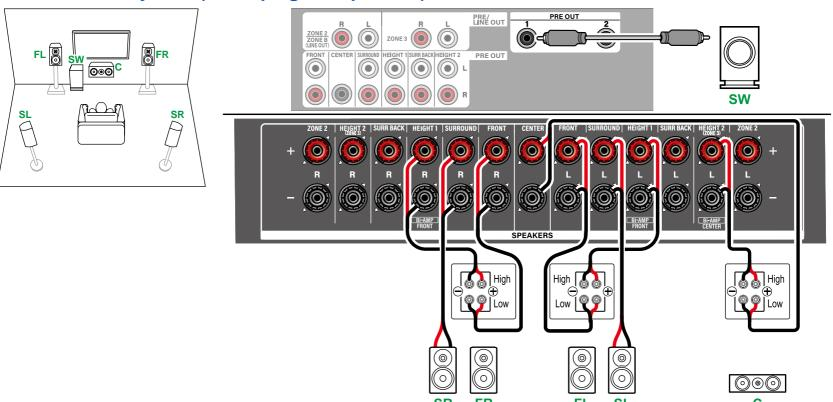
Be sure to remove the jumper bar connecting between the woofer jacks and tweeter jacks of the Bi-Amping supported speakers. Refer to the instruction manual of your speakers as well.
