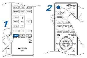
"Z2" lights in the main unit display when ZONE 2 turns on. To turn ZONE 2 off, repeat the same procedure.
