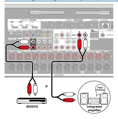
You can enjoy 2 ch audio in the separate room (ZONE 3) while performing playback in the main room (where this unit is located). Use an analog audio cable to connect the ZONE 3 PRE/LINE OUT jack on this unit to the input jack on an integrated amplifier in the separate room. The same source can be played back in the main room and ZONE 3 simultaneously. Also, different sources can be played back in both rooms.
