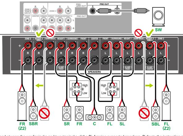
Be sure to remove the jumper bar connecting between the woofer jacks and tweeter jacks of the Bi-Amping supported speakers. Refer to the instruction manual of your speakers as well.
