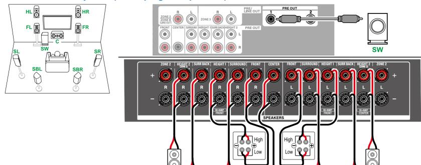
Be sure to remove the jumper bar connecting between the woofer jacks and tweeter jacks of the Bi-Amping supported speakers. Refer to the instruction manual of your speakers as well.
