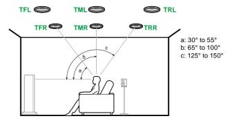
TFL, TFR Fit top front speakers on the ceiling in front of the listening position.
