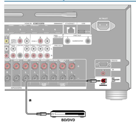
When connecting a device equipped with a 12V TRIGGER IN jack such as a BD/DVD player to this unit, the device can be turned on or set to standby by interlocking the operation on this unit. When the desired input is selected on the unit, power link operation will be activated with a control signal of maximum 12 V/100 mA from the 12V TRIGGER OUT jack.
