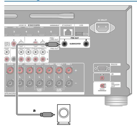
Connect a powered subwoofer with this unit using a subwoofer cable. Up to two powered subwoofers can be connected.
