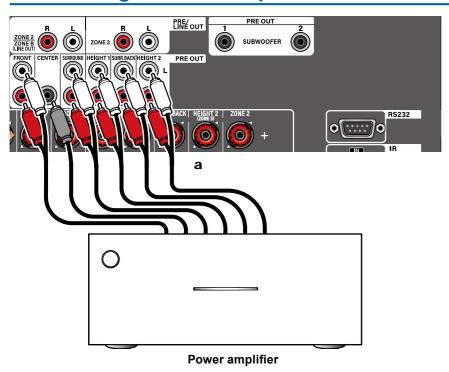
You can connect a power amplifier to the unit and use the unit as a pre-amplifier. Use an analog audio cable for connection.
