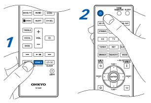
"Z3" lights in the main unit display when ZONE 3 turns on. To turn ZONE 3 off, repeat the same procedure.
