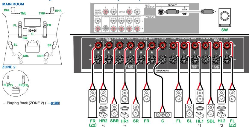
• While ZONE 2 playback is being performed, surround back speakers installed in the main room cannot play audio.
