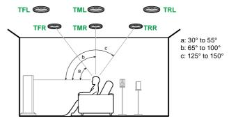
TFL, TFR Fit top front speakers on the ceiling in front of the listening position.
