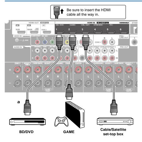
This is a connection example of an AV component equipped with an HDMI jack. When connecting with an AV component that conforms to the CEC (Consumer Electronics Control) standard, you can use the HDMI CEC function (\*) that enables linking with input selectors, etc. and the HDMI Standby Through function that can transmit video and audio signals of the AV component to the TV even if this unit is in standby mode.
