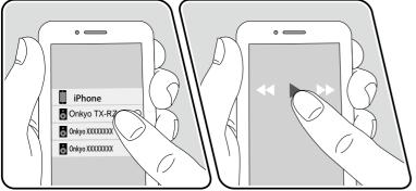
This unit supports AirPlay2. If the version of the iOS device is iOS11.4 or later, you can play the tracks on the iOS device simultaneously on this device and on another device that supports AirPlay2.
