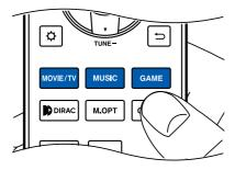
2. Press the selected button repeatedly to switch the modes displayed on the display of the main unit.
