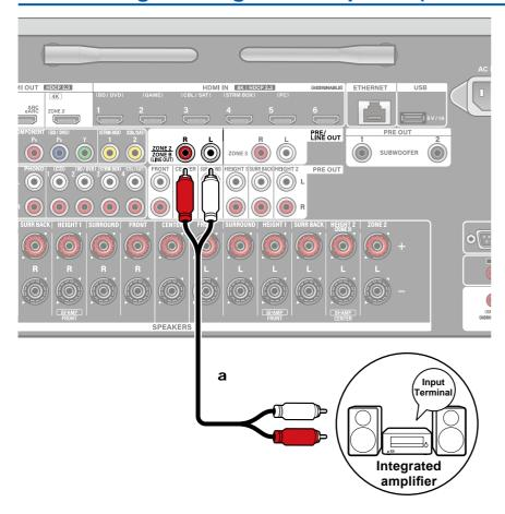
You can enjoy 2 ch audio in the separate room (ZONE 2) while performing playback in the main room (where this unit is located). Use an analog audio cable to connect the ZONE 2 PRE/LINE OUT jacks on this unit to the input jack on an integrated amplifier in the separate room.
