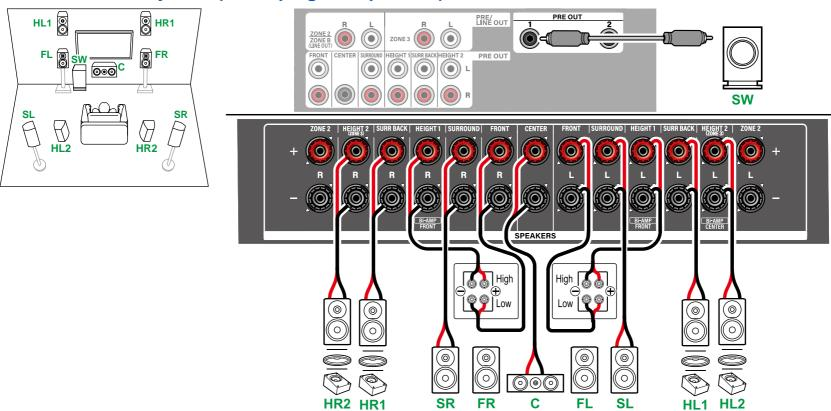
Be sure to remove the jumper bar connecting between the woofer jacks and tweeter jacks of the Bi-Amping supported speakers. Refer to the instruction manual of your speakers as well.
