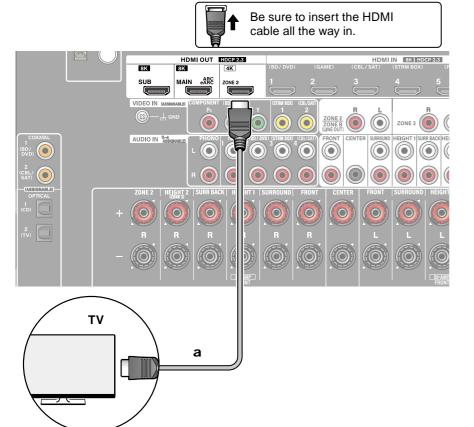
While a disc is played on a Blu-ray Disc player in the main room (where this unit is located), you can play the video and audio of the same Blu-ray Disc player or another AV component on the TV equipped with an HDMI IN jack in a separate room (ZONE 2).
