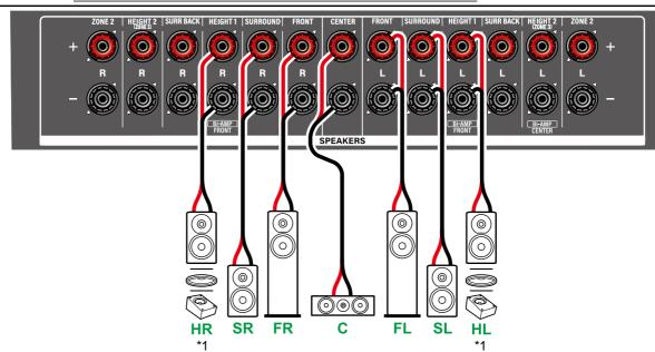
\*1 Connect the Height Speakers you have actually installed (HL/HR: Height Speakers, Top Speakers, Dolby Enabled Speakers).
