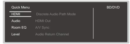
You can make the settings on the TV screen during playback. Press Q on the remote controller to display the Quick Menu.
