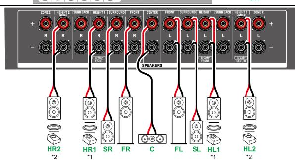
\*1 Connect the Height Speakers you have actually installed (HL1/HR1: Front Height Speakers, Top (front side) Speakers, Dolby Enabled Speakers (Front)).
