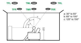
**TFL**, **TFR** Fit top front speakers on the ceiling in front of the listening position. **TML**, **TMR** Fit top middle speakers on the ceiling directly above the listening
