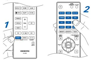
• Information of a connected device can be displayed on the TV screen in the separate room. While pressing and holding the ZONE 2 HOLD button on the remote controller, press the " i " button.
