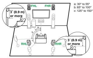
FHL, FHR Place the front high speakers directly above the front speakers, angled to face the listening position.
