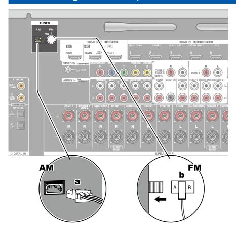
Connect the antenna to this unit, and set up the antenna at the best position for listening while receiving radio signals. Attach the indoor FM antenna to the wall using push pins or adhesive tape.
