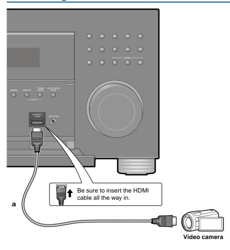
Connect a video camera, etc. to the AUX INPUT HDMI jack on the front panel using an HDMI cable.
