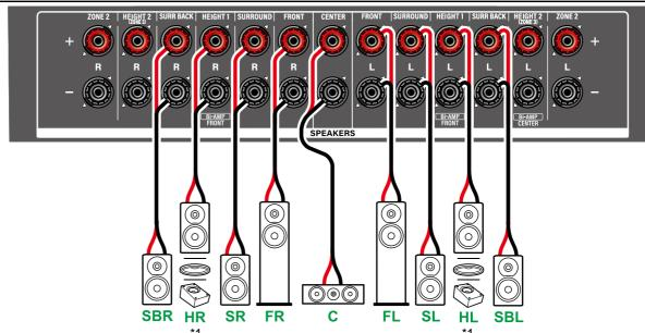
\*1 Connect the Height Speakers you have actually installed (HL/HR: Height Speakers, Top Speakers, Dolby Enabled Speakers).
