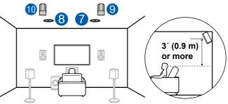
The width between the rear high speakers should match the one for the front speakers, and they should be installed minimum of 3'/0.9 m higher than the front speakers, and tilted so they will point toward the listener.
