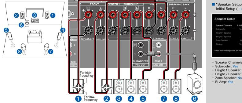
You can configure a 7.1 Channel System ( $\rightarrow p15$ ) by connecting front speakers that support Bi-Amping connection. The Bi-Amping connection can improve the quality of the low and high pitched ranges. Be sure to remove the jumper bar connecting between the woofer jacks and tweeter jacks of the Bi-Amping supported speakers. Refer to the instruction manual of your speakers as well.
