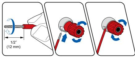
Make correct connection between the unit's jacks and speaker's jacks (+ side to + side, and - side to - side) for each channel. If the connection is wrong, a bass sound will not be reproduced properly due to reverse phase. Twist the wires exposed from the tip of the speaker cable so that the wires do not stick out of the speaker terminal when connecting. If the exposed wires touch the rear panel, or the + side and – side wires touch each other, the protection circuit will be activated.
