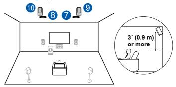
The width between the rear high speakers should match the one for the front speakers, and they should be installed minimum of 3'/0.9 m higher than the front speakers, and tilted so they will point toward the listener.
