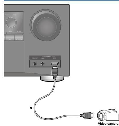
Connect a video camera, etc. to the AUX INPUT AUDIO/HDMI jack on the front panel using an HDMI cable or stereo mini plug cable ( $\emptyset$ 1/8"/3.5 mm).
