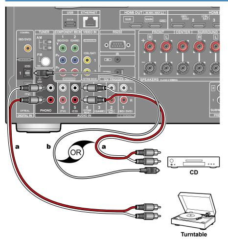
This is a connection example of an audio component. Connect a CD player using a digital optical cable or analog audio cable. You can also connect a turntable that has an MM-type cartridge to the PHONO jack.
