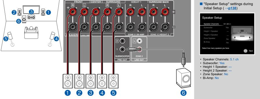
This is a basic 5.1 Channel System. For details of the speaker layout, refer to "Speaker Installation" ( $\rightarrow p14$ ).
