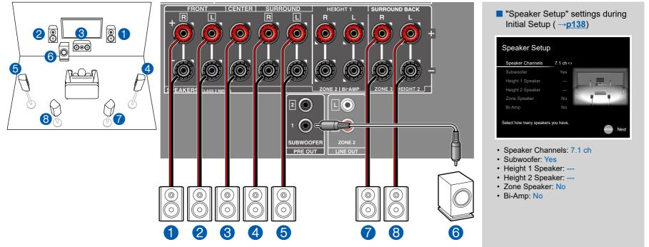
This is a 7.1 Channel System that consists of the basic 5.1 Channel System and added surround back speakers. For details of the speaker layout, refer to "Speaker Installation" ( $\rightarrow p15$ ).
