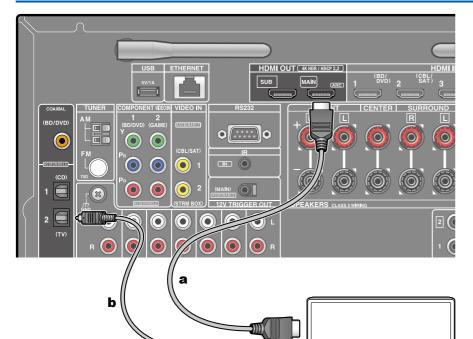
If the TV does not support the ARC (Audio Return Channel) function (\*), connect an HDMI cable and digital optical cable. If the TV does not have a DIGITAL OPTICAL OUT jack, you can use an analog audio cable to connect with the AUDIO IN TV jack.
