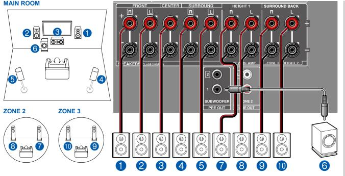
**MAIN ROOM:** This is a basic 5.1 Channel System. For details of the speaker layout, refer to "Speaker Installation"  $(\rightarrow p14)$ .
