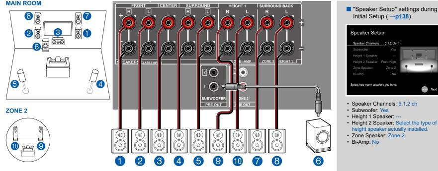
**MAIN ROOM:** This is a combination of the 5.1 Channel System and front high speakers. A front high speaker is a type of height speaker. You can select only one set of height speakers from the following three types for connection.
