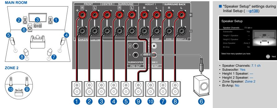
**MAIN ROOM:** This is a 7.1 Channel System that consists of the basic 5.1 Channel System and added surround back speakers. For details of the speaker layout, refer to "Speaker Installation" ( $\rightarrow p15$ ).
