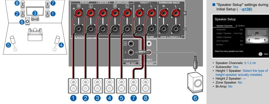
This is a combination of the 5.1 Channel System and front high speakers. A front high speaker is a type of height speaker. You can select only one set of height speakers from the following three types for connection.
