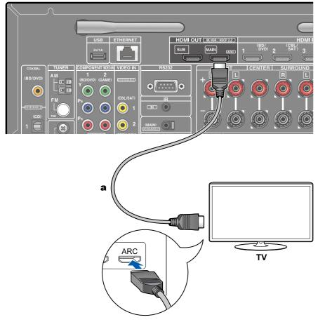
If the TV supports the ARC (Audio Return Channel) function (\*), use only the HDMI cable to connect with the TV. Use the ARC-compatible HDMI IN jack of the TV for connection.
