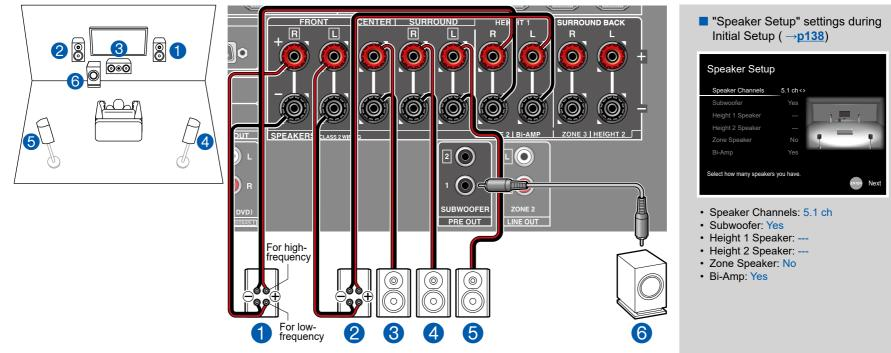
You can configure a 5.1 Channel System ( $\rightarrow$ **p14**) by connecting front speakers that support Bi-Amping connection. The Bi-Amping connection can improve the quality of the low and high pitched ranges. Be sure to remove the jumper bar connecting between the woofer jacks and tweeter jacks of the Bi-Amping supported speakers. Refer to the instruction manual of your speakers as well.
