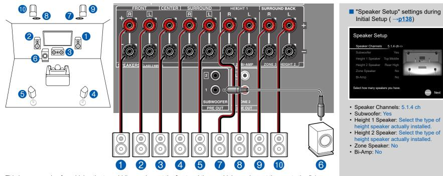
This is an example of combining the top middle speakers at the front and the rear high speakers at the rear to the 5.1 Channel System. The height speakers in front can be selected from following 4 types. The height speakers that can be combined at the rear differ depending on the height speakers used at the front.
