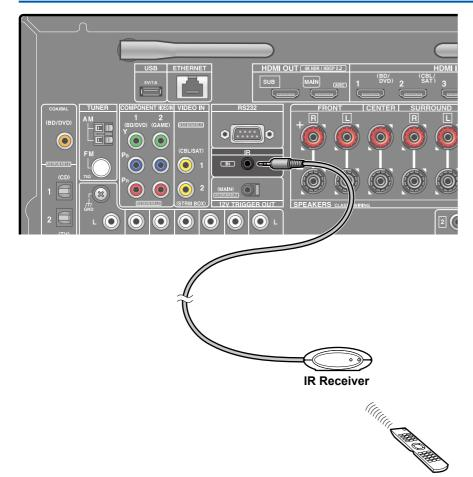
When connecting a remote control receiver unit consisting of an IR Receiver, etc. to this unit, operation using the remote controller is possible even if the remote control signal is difficult to reach (due to installation in the cabinet, etc.). You can also operate the unit using the remote controller from a separate room such as ZONE 2. For adopting a remote control receiver unit, contact the specialized stores.
