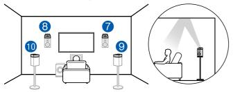
The Dolby enabled speakers are the special speaker that the sound is emitted toward the ceiling, and have the effect the sound to come from above by reflecting the sound on the ceiling.
