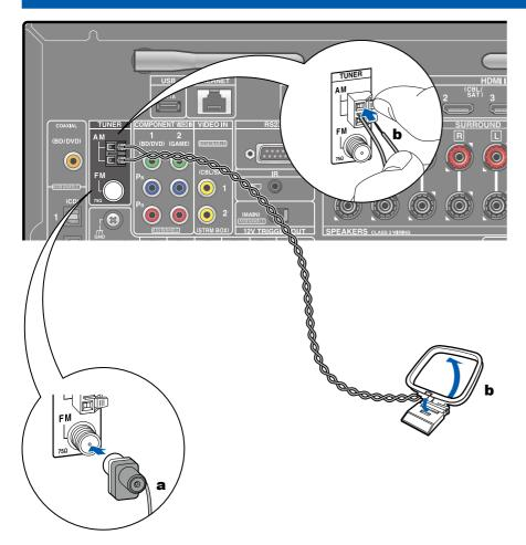
Connect the antenna to this unit, and set up the antenna at the best position for listening while receiving radio signals. Attach the indoor FM antenna to the wall using push pins or adhesive tape.
