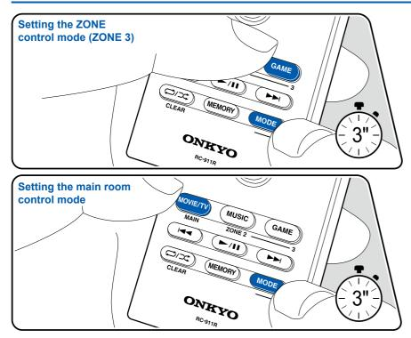
At the time of purchase, the remote controller is in the mode to control playback in the main room. Settings are required to playback a source in ZONE 3. Set "2.Speaker" - "Configuration" - "Zone Speaker" in the Setup menu ( $\rightarrow$ p113) to "Zone 2/Zone 3", and set the remote controller to the ZONE control mode (ZONE 3). To control the main room play again, restore the remote controller to the main room control mode.
