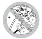
Make sure the exposed speaker cables do not stick out of the speaker terminals when connecting. If the exposed wires of the speakers touch the rear panel or the + and – wires touch each other, the protection circuit will be activated.
