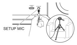
When putting the speaker setup microphone on a tripod, refer to the illustration when putting it in place.
