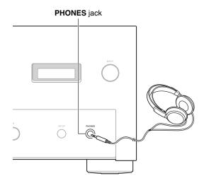
**1** Connect a pair of stereo headphones with a standard plug (1/4 inch or 6.3 mm) to the PHONES jack.
