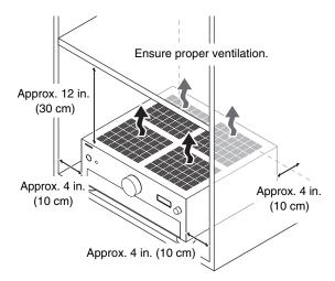
Install the integrated amplifier on a sturdy rack or shelf. Position it so that its weight is evenly dispersed on its four legs. Do not install the integrated amplifier in a place with vibration or an unstable location.
