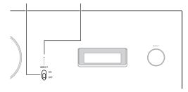
**1** Set the DIRECT switch to the ON position. The information display goes off and the DIRECT LED lights.
