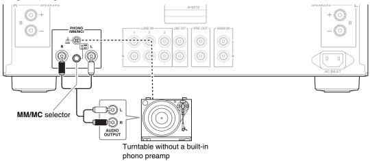
Use the **MM/MC** selector on the back of the integrated amplifier to select either **MM** or **MC**, in accordance with the cartridge format of the turntable.
