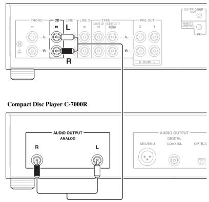
This is an example of analog connection using the preamplifier P-3000R.
