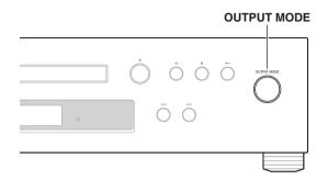
Switch the output between DIGITAL/ANALOG, DIGITAL, ANALOG in order.
