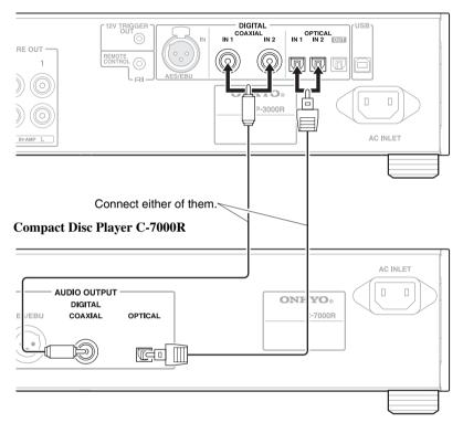
This is an example of digital connection using the preamplifier P-3000R. Connect either of them.
