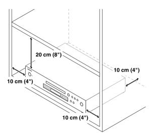
Install the compact disc player on a sturdy rack or shelf. Position it so that its weight is evenly dispersed on its four legs. Do not install the compact disc player in a place with vibration or an unstable location.
