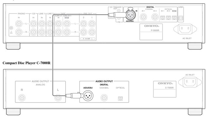
This is an example of AES/EBU connection using the preamplifier P-3000R.
