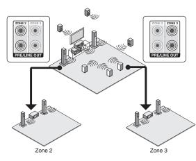
Volume can be adjusted with both the unit and the integrated amplifier used in a separate room. To adjust it with the unit, press RECEIVER and then HOME on the remote controller, select "Setup" - "7. Hardware Setup" -"Multi Zone" - "Zone 2 Out" or "Zone 3 Out" and set the setting to "Variable". If you connect a power amplifier, be sure to make the setting and adjust the volume in the main room.
